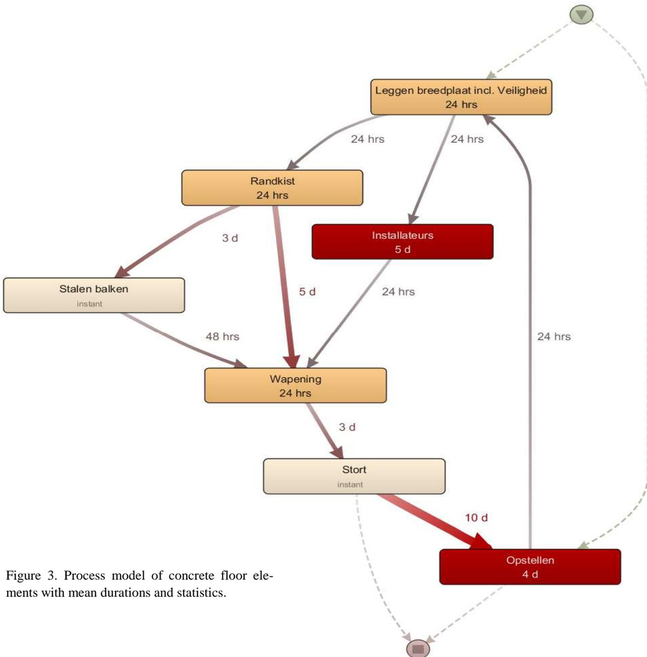
Figure 3. Process model of concrete floor elements with mean durations and statistics.
