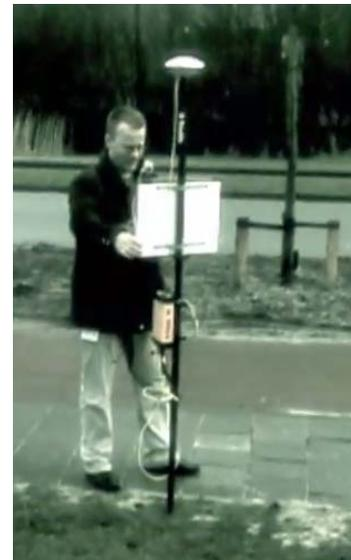
Note that this system does not deliver the same accuracy in all directions. In the horizontal range it is less than 1 meter. In the vertical range it is less than 5 meters (according to the supplier Trimble). This is a significant shift for actual buildings. Therefore some kind of calibration has to be carried out with a basic reference object in reality that overlaps with an object in virtual reality.
